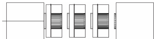
图 9 副油缸推进卸饼过程仿真结束位置 Fig. 9 End position of simulation of auxiliary cylinder pushing and unloading cake process
